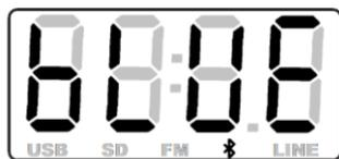
Pressing the mode button until the display shows "bLUE" enters Bluetooth receiver mode.
