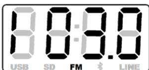
Pressing the mode button until "FM" appears in the lower part of the display enters FM tuner mode.
